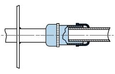
For vertical mount with weight suspended from Quik-Joint, use Safe-T Nut to prevent pipe from pulling out. See below.
