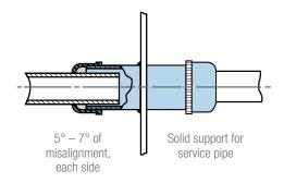
Complete Quik-Joint on welded pipe nipple. For disassembly, allow Quik-Joint to slide toward wall enough to clear opposite service pipe. Provides maximum misalignment.
