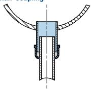
Connect to round tanks, manifolds, reservoirs, headers by boring a hole, inserting Quik-Joint half-body and welding in place.
